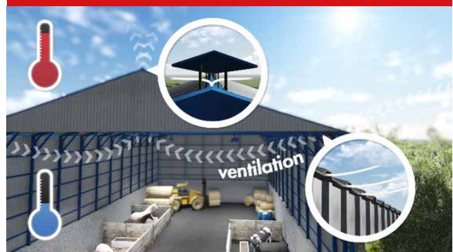
Ventilation is key to keep the building dry
