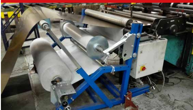
Lantor applicators for factory processing
